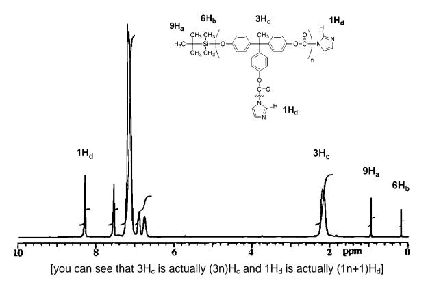
2. For the polycarbonate structure and <sup>1</sup>H NMR spectrum given:
